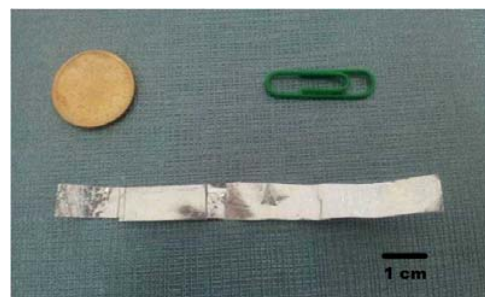
Figure 2. Bimorphs of electroded PVDF sheets
