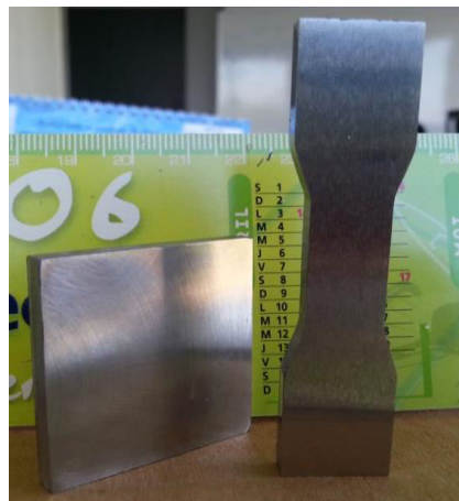
Figure: Complex shape samples consolidated by Spark Plasma Sintering.
