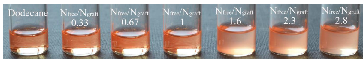
Figure1. The QDs dispersed in silicone with different polymer chain length
